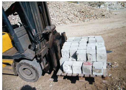
Fig. 1. Concrete specimens after compression test going to be recycled for new aggregates
