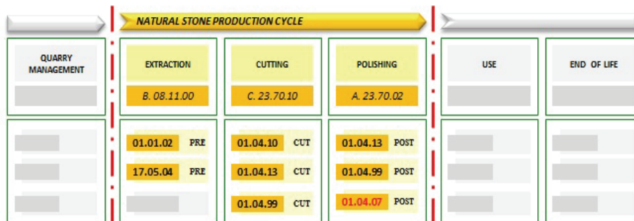
Fig. 4. Natural stone production cycle (level 1) - subdivision of a typical supply chain in “manufacturing stages”
