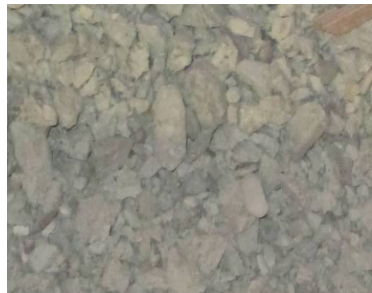
Fig. 2. Recycled concrete aggregates after crushing
